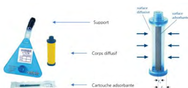
Figure 26 : Echantillonneur passif Radiello
